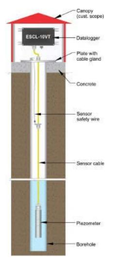
Typical installation scheme for automatic groundwater monitoring system
