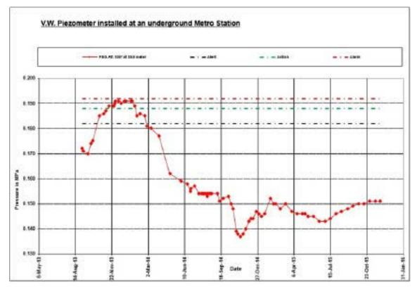
Sample data from vibrating wire piezometer
