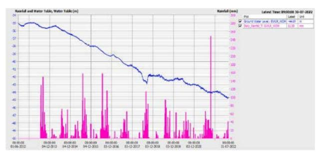
Online groundwater level and rainfall data from a factory in Lucknow. It is observed that water level increases a little after each monsoon. Yet it has recorded long-term water level decline with almost same amount of rainfall, due to extensive groundwater use.
