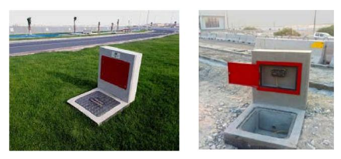
Piezometers installed with dataloggers at different construction sites
